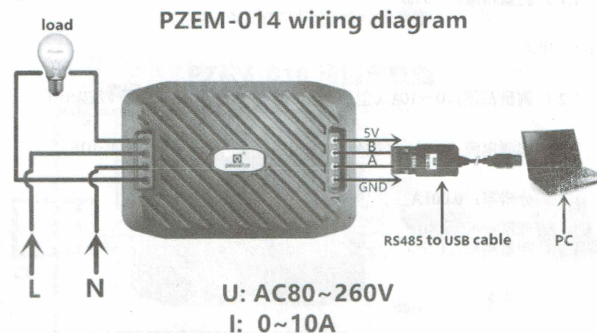
Picture 4.1 PZEM-014 wiring diagram
